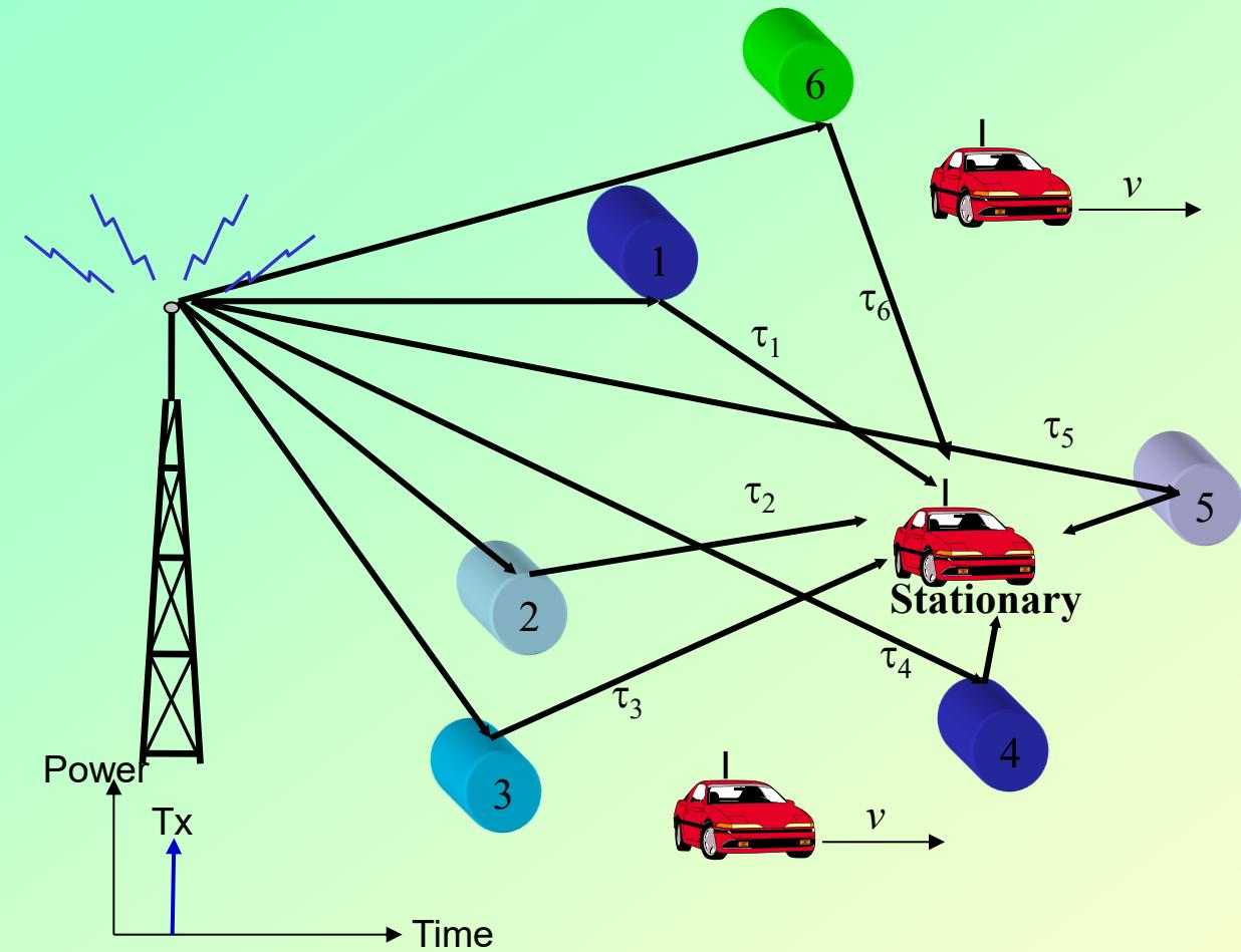
The maximum delay for which the received power level becomes negligible is known as the **maximum delay spread**  $\tau_{\max}$ . Sometimes Root-Mean-Square value  $\tau_{\text{rms}}$  is used.
