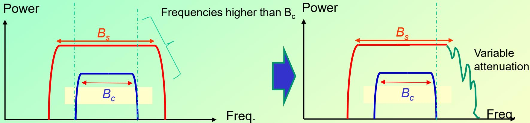
Thus, Variable attenuation outside the BC band leads to signal distortion  $\rightarrow$  Frequency selective fading
