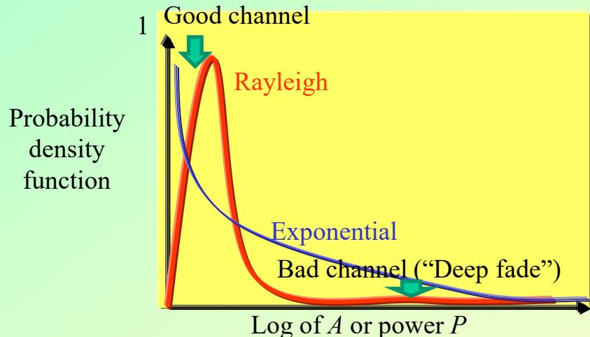
Which is Rayleigh distributed: Assuming all components received have approximately the same power and that all are resulting from scattering.
