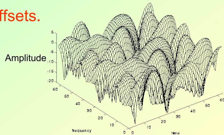
Channel amplitude in dB versus location (= time\*velocity) and frequency
