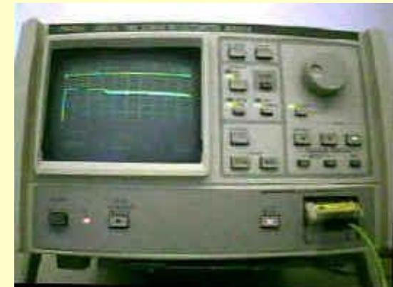
Attenuation along the fibre link can be measured using **Optical Time Domain Reflectometer**
