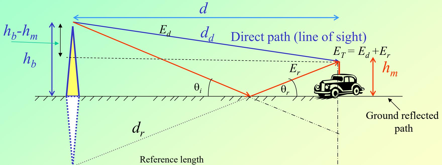
$$E_{d_d}(d, t) = \frac{E_o d_o}{d_d} \cos \left( w_c \left( t - \frac{d_d}{c} \right) \right) \quad E_{d_r}(d, t) = \rho \frac{E_o d_o}{d_r} \cos \left( w_c \left( t - \frac{d_r}{c} \right) \right)$$
