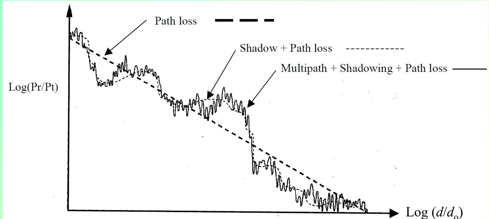
$$P_r [\text{dBm}] = P_t [\text{dBm}] + \text{path loss} [\text{dB}] + \text{shadowing} [\text{dB}] + \text{multipath} [\text{dB}]$$
