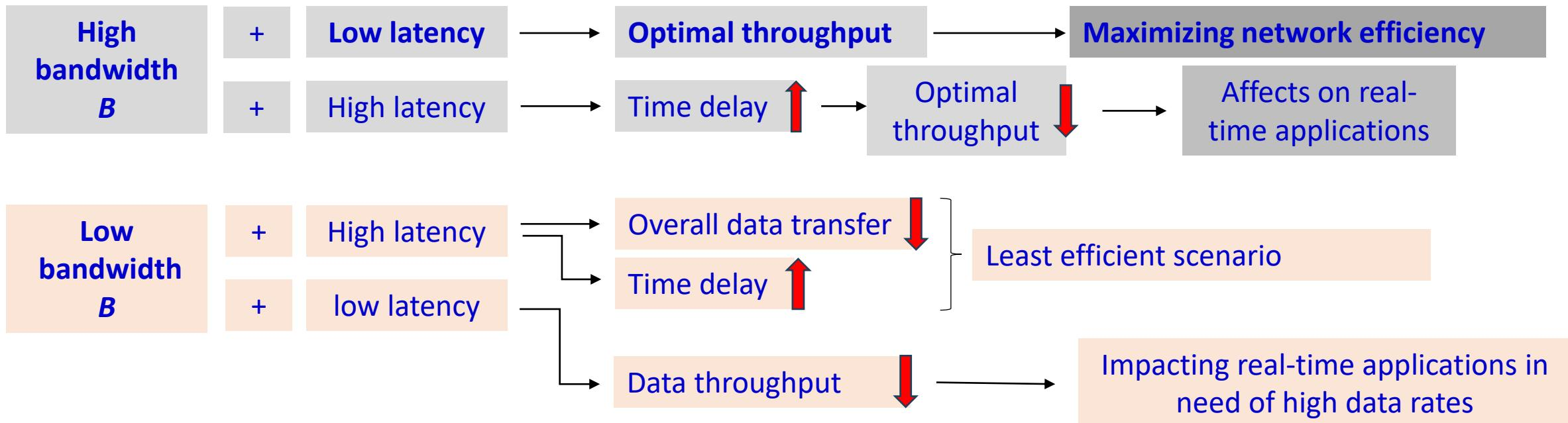
$$\text{Throughput } R_{\text{Th}} = B \text{ [Hz]} \cdot D \text{ [cell/km}^2\text{]} \cdot \eta_{\text{sp}} \text{ [bit /s /Hz / cell]}$$
